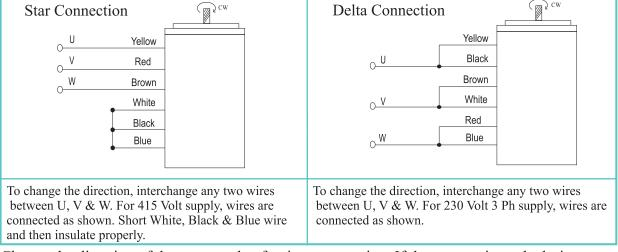
Change the direction of the motor only after it stops rotating. If the attempt is made during rotation, motor may ignore the reversing command or change the direction after some time.
